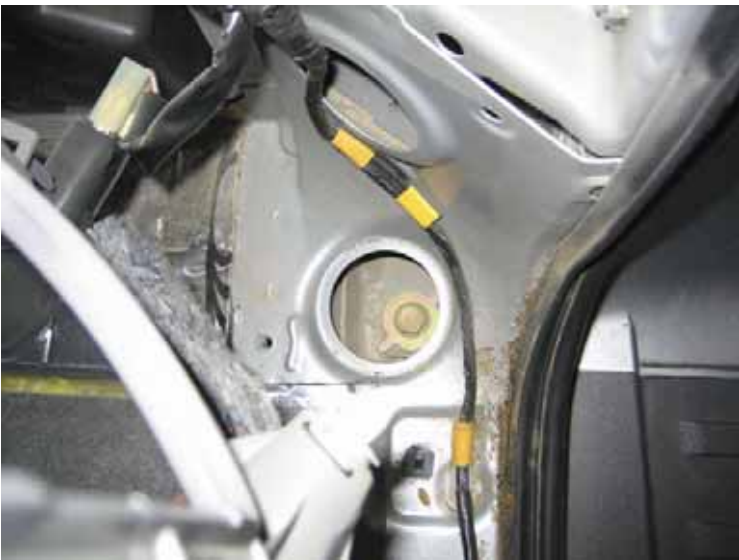
Rear cabin trim and body mounts. These mounts are just in front of the rear wheel well.
