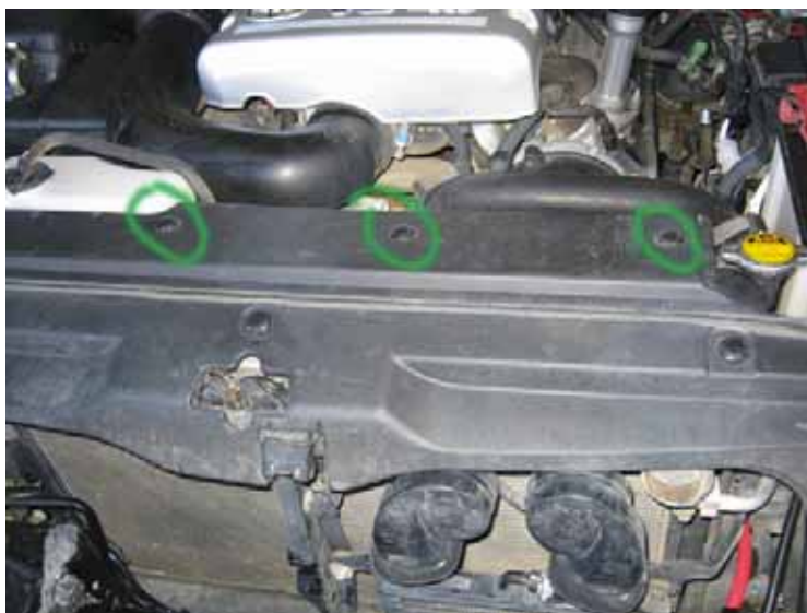
It will also help to remove the radiator top trim piece by unclipping the 11 plugs that hold it place. Pics below.
