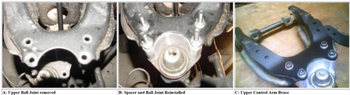
A: Upper Ball Joint removed
