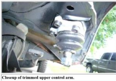
Closeup of trimmed upper control arm.
