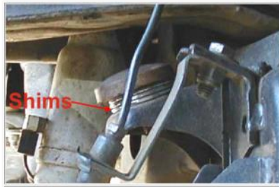
Shimming for low profile bump stops
