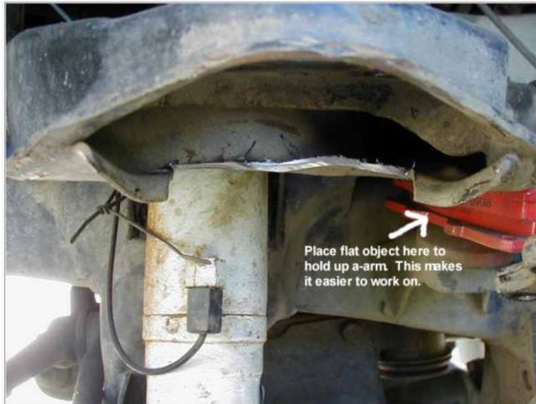
Trimming around upper ball joint
