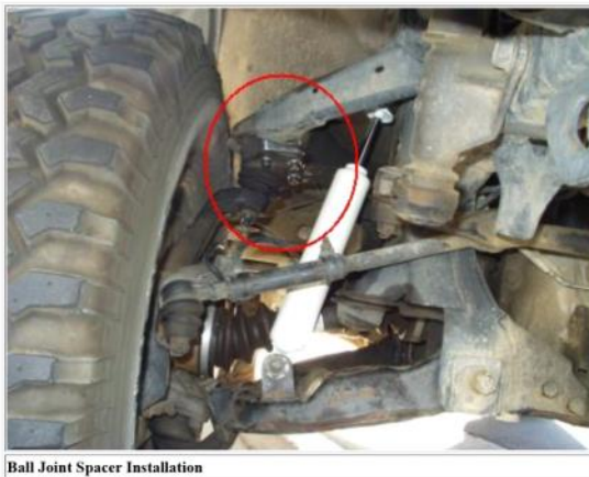
Ball Joint Spacer Installation
