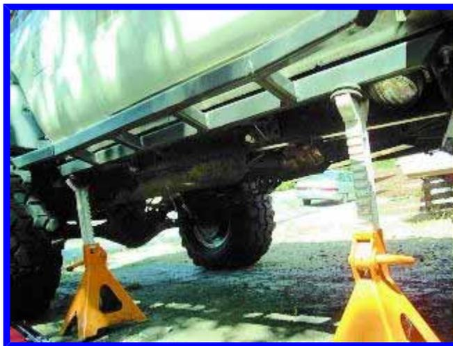
I was able to install these bars by myself, using a pair of jack stands and scraps of wood to position the bars in the correct location. If you have a few helpers, have someone hold each end of the bar in position, roughly centered between the wheel wells and roughly parallel to the body seam. You may need to move the bars back and forth and up and down a bit to find where they fit the frame and body best. The fit of the bars to the frame and body is what matters.
