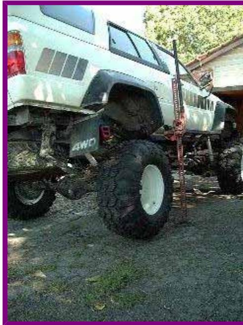
The outer bar is supported by outriggers off the inner bar and it is offset about 2" higher and lines up just a bit outside the widest part of the body. This offers protection of the body panel from vertical obstructions while maximizing ground clearance under the bars.
